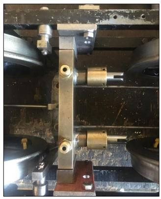
The twin pump was donated by a club member. It had originally been destined for a 5inch gauge B1. As can be seen in the photo's the pump was made to also act as a frame stretcher.
